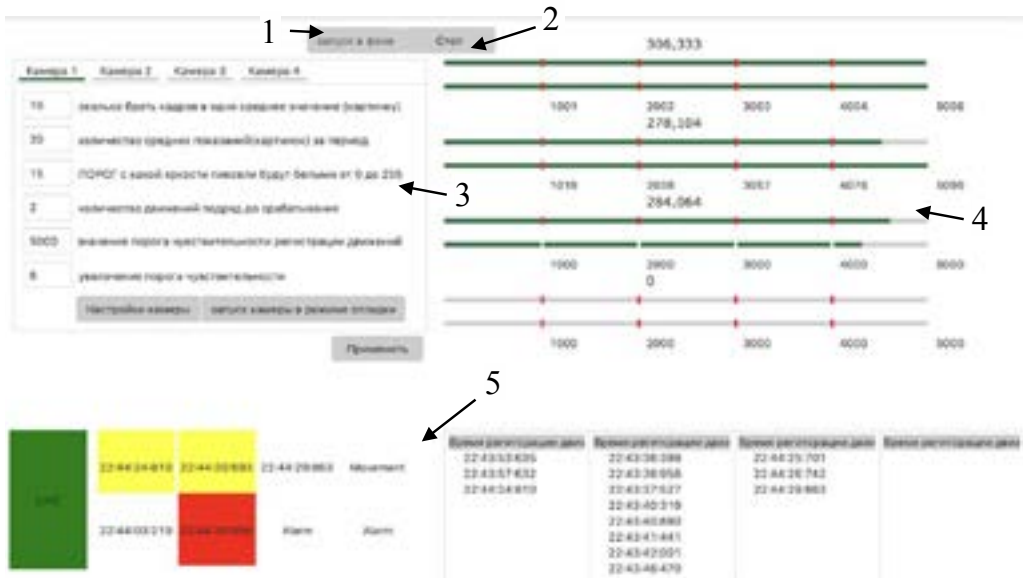
1 - "start in background" button; 2 - "stop" button; 3 - block "settings"; 4 - block of "devices for displaying measured values"; 5 - block "signaling and sending messages".
