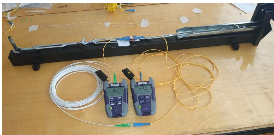
Figure 1 – Laboratory sample of a fiber optic pit wall displacement sensor
