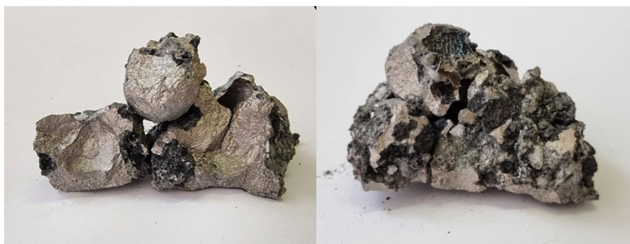
I Alloy melting charge No. II Alloy melting charge No. Figure 5-shows samples of the production of ferroalloys
