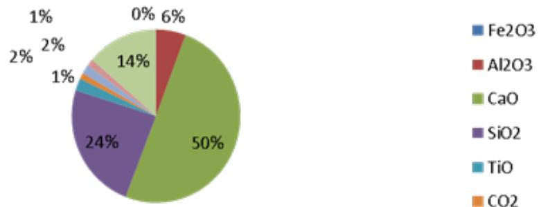
Figure 1 – Chemical composition of bauxite sludge
