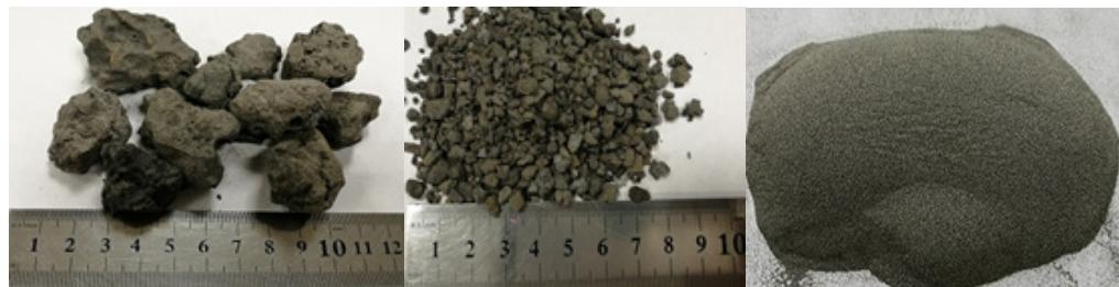
Figure 3 – Metallurgical slag of Pavlodar enterprises
