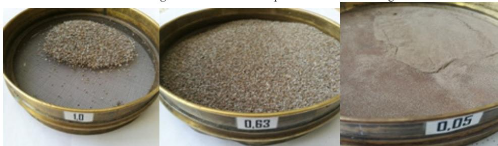
Figure 2 – Granulometric analysis of bauxite sludge
