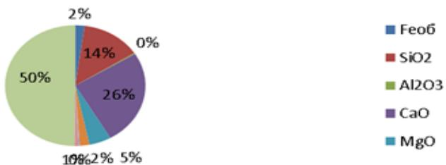
Figure 4 – Average chemical composition of metallurgical slag of Pavlodar
