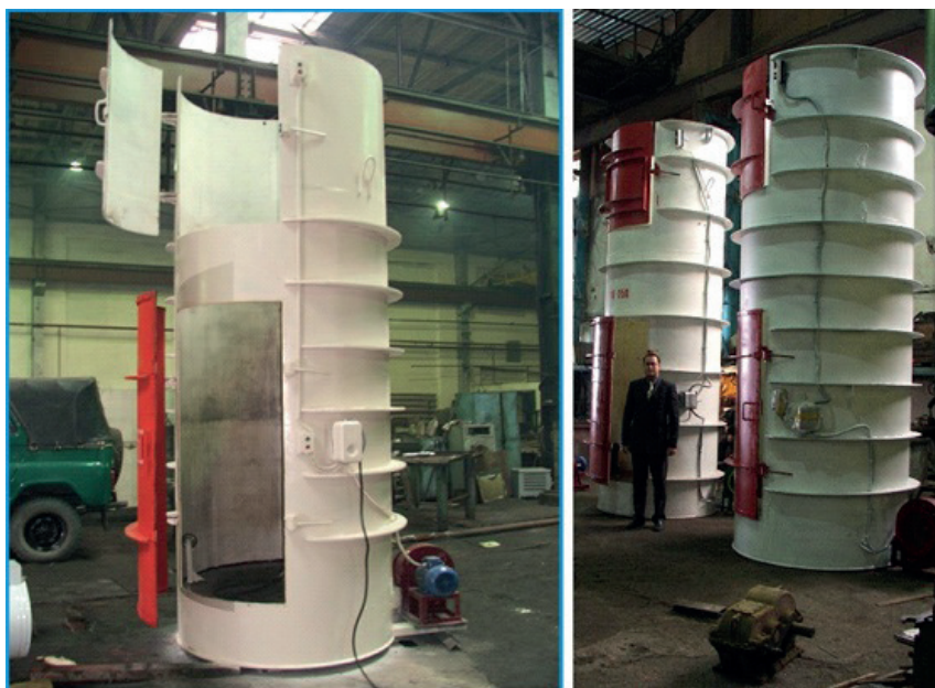
Figure 1 - Three modifications of load pneumatic hoists with the lifting capacity of 110, 250 and 500 kg
