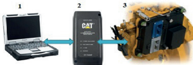
Fig. 3. Location of connection of elements of the BEU system: 1 - service computer with CAT software; 2 - adapter connecting the engine ECM and the computer; 3 - electronic control unit ECM
