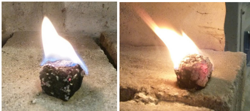
Figure 5. The process of combustion of a briquette made of Coal of the Kiyakty deposit with a ARPD binder
