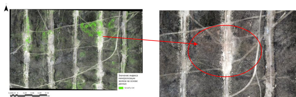
Figure 2 – Results of UAV Data Processing Highlighting the Area with Iron Oxide Concentration
