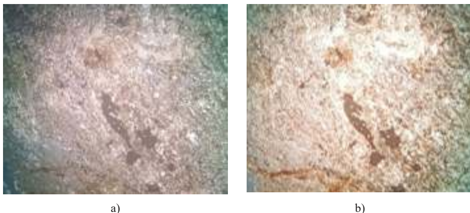
Figure 4. Sericitic schists and the ore minerals contained within them (black dots). Thin section №5. Magnification 25x: a) without analyzer, b) without analyzer.
