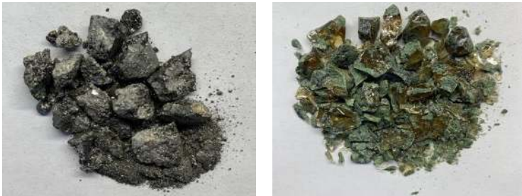
Figure 6. Products of high-carbon ferromanganese smelting: (a) alloy, (b) slag.
