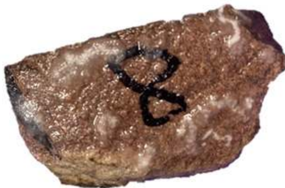
Figure 4. Secondary Precipitation on the Rock Surface Induced by Treatment with an HF-Containing Acid System.
