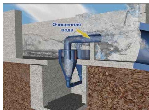
Figure 2 – General view of the developed hydrocyclone sand trap
