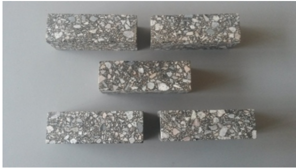
Figure 2 – Samples of the asphalt concretes and polymer asphalt concretes with dimension 5x5x16 cm to be tested
