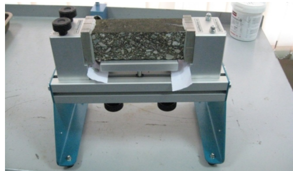
Figure 5 – The asphalt concrete sample with glued metal plates in a specially assembled installation
