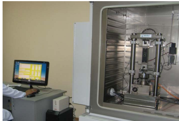
Figure 7 – The asphalt concrete sample under test in a thermal chamber of TRAVIS
