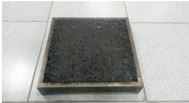
Figure 4 – A square slab of asphalt concrete with dimension 5x30.5x30.5 cm
