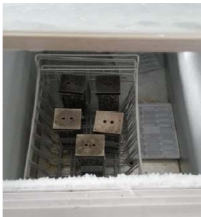
Figure 6 – The asphalt concrete samples in a freezing chamber
