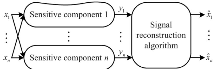
Figure 1 – Schematic structure of a multifunctional sensor [10]
