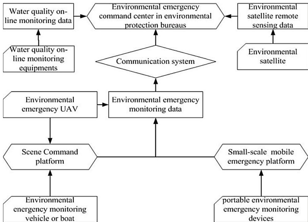
Figure 2 – Structure of water environmental monitoring network based on space-earth integration system [13]
