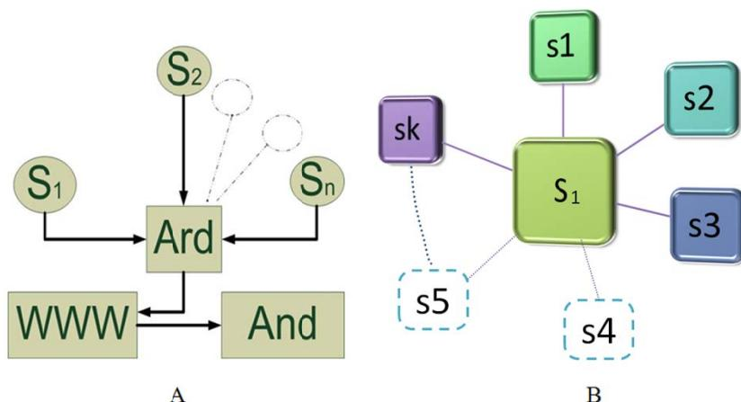
WWW – World Wide Web; Ard – Arduino uno; And – Android app; S<sub>1</sub>, S<sub>2</sub>, S<sub>3</sub>... S<sub>n</sub> – multifunctional sensors; s1, s2, s3, s4, ... sk – sensors.
