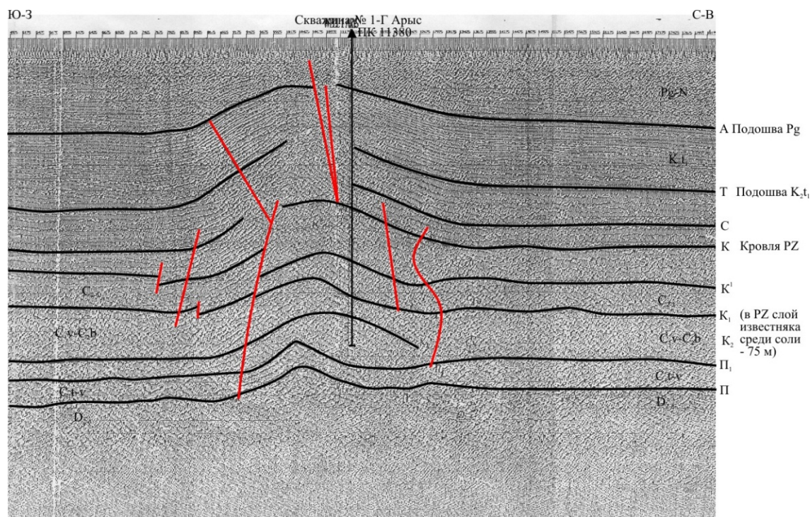
Figure 2 – Fragment of the seismic profile No. 9207170, intersecting the Arys dome structure (by N. G. Davydov)
