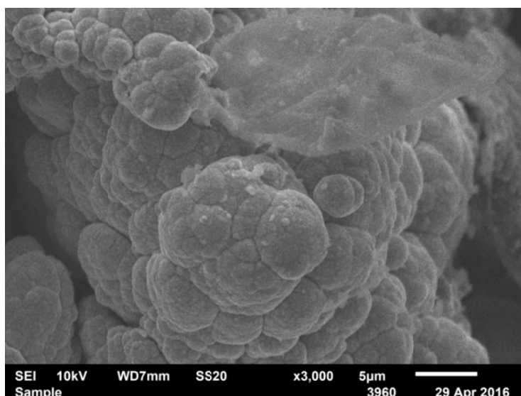
Figure 2 – A microphotograph of a gray nickel powder produced at polarization with impulse cathodic current in an ultrasonic field at a frequency of 35 kHz
