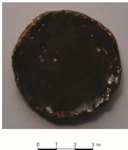
Figure 6 – Photo illustrations of the burned dacite product. The temperature and chronological parameters of burning under high-temperature heating conditions of 1400 °C (5', 50', 30'), sample K-12-15
