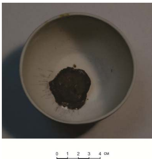
Figure 4 – Photo illustrations of the gabbro-amphibolite calcination product. The temperature-chronological parameters of roasting under high-temperature heating conditions are 1400 °C (5', 30', 20'), sample K-13-15
