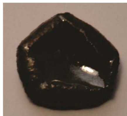
Figure 3 – Photographic illustration of the burned product of the Saga basalt suite. The temperature and chronological parameters of burning under high-temperature heating conditions of 1400 °C (5', 50', 30'), sample K-14-15-2
