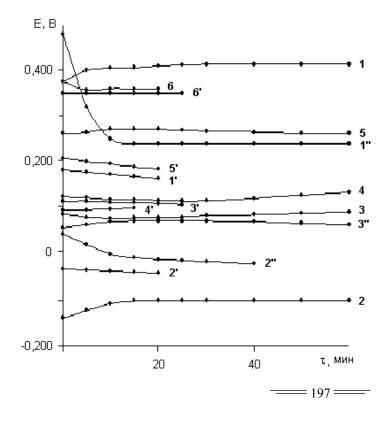
$Figure 1 - \\ Potential-time dependences of RPWE (1-6), \\ RE (1'-6'), RPSUE (1 "-3") \\ in 0.1N solutions of electrolytes \\ 1-1" - H_2SO_4; \\ 2-2" - KSCN; \\ 3-3" - KCl; \\ 4, 4' - HCl; \\ 5, 5' - H_3 PO_4; \\ 6, 6' - H_2SO_4 + 1.68 \cdot 10^{-2} \, N \, HgSO_4 \\ \end{cases}$
