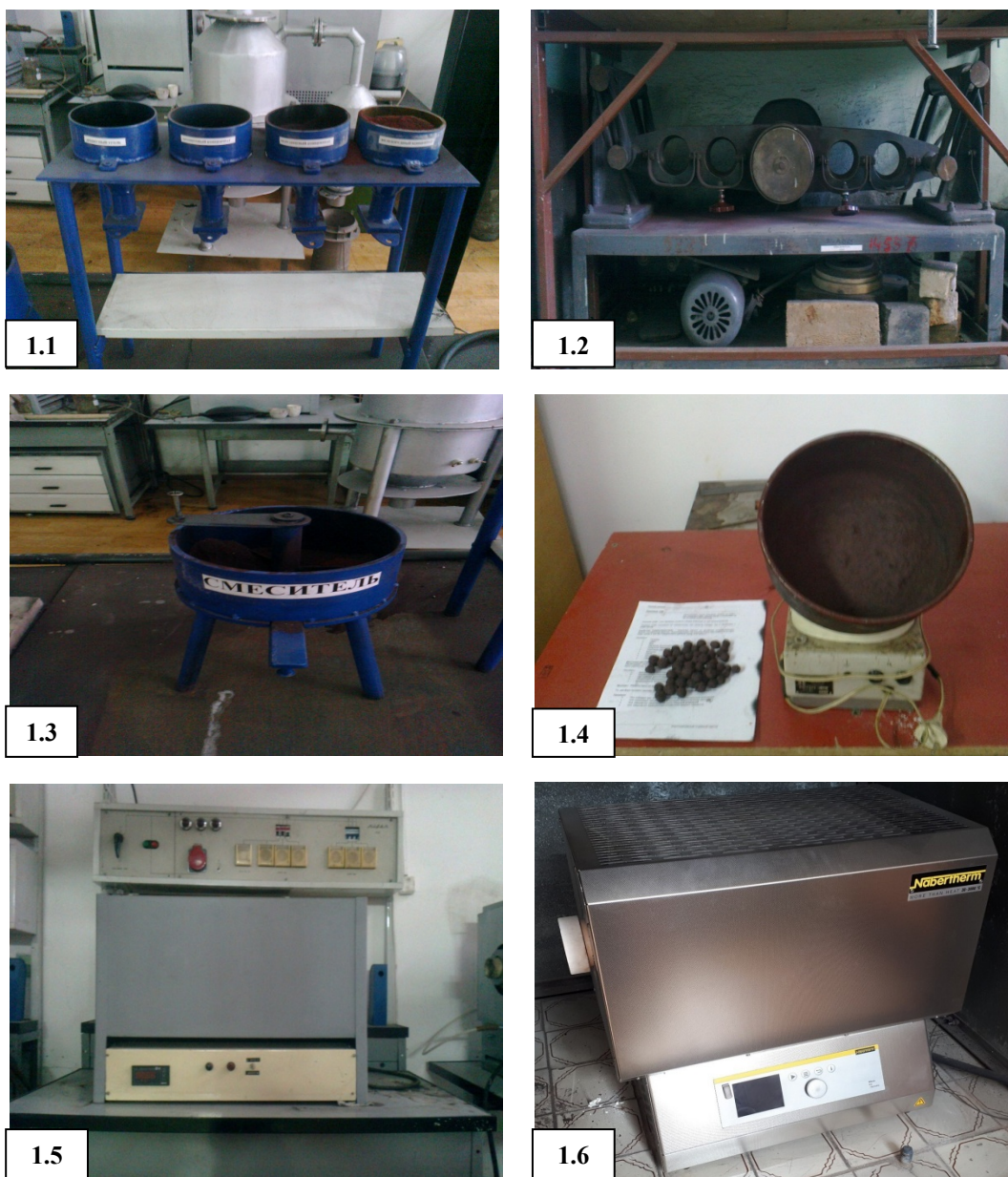
Figure 1 – Lab equipment and apparatus: 1.1 - bunkers for charge components; 1.2 – Electric-vibrating cutting machine; 1.3 – batch blending system; 1.4 - charge granulator; 1.5 - oven «SUOL-044 12-M2» for metallization; 1.6 - smelt furnace «RHTC 80 - 230/15 Controller B410»
