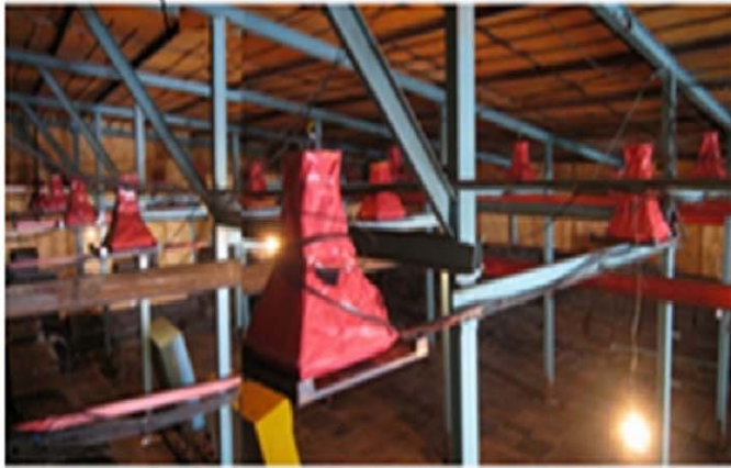
Figure 1 – Scintillation detectors installed in the launch building
