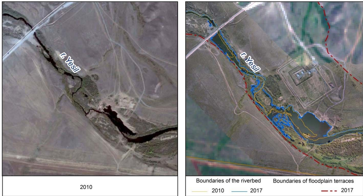
Figure 6 – Anthropogenic changes in the bed and floodplain of the river Yesil near Volgodonovka village, for 2010 and 2017 with the formation of lake-shaped extensions at the places of development of common minerals
