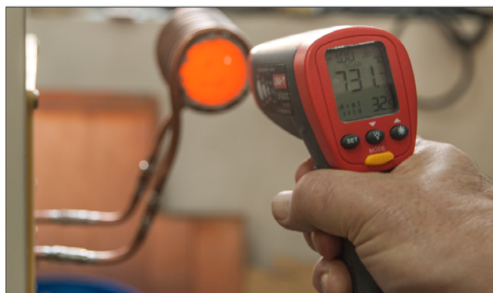
Figure 4 – The process of induction heating of metal to a temperature of 731 0 C
