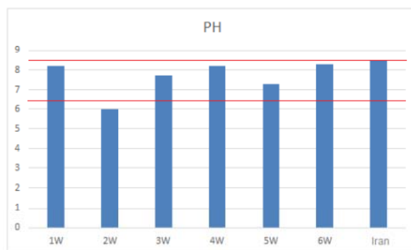
Chart 1 – PH concentration chart of water samples and comparison with Iranian Standard
